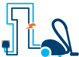
Parallel Arc Fault
